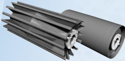
PPI (Precision Pulley & Idler) Pulleys utilizing the extra wide XT hubs, XT bushings, and heavy end discs give the best transfer of torque from the drive to the conveyor belt load. Head pulleys have 3/8 inch herringbone lagging— standard. Winged tail pulleys provide longer belt life by being self cleaning, keeping material from lodging between belt and pulley.
