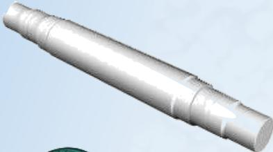
FAB TEC conveyor shafts are manufactured from TG&P (turned, ground, and polished) C1045 (82,000 psi tensile strength) medium carbon steel for superior strength, toughness, and machinability.
